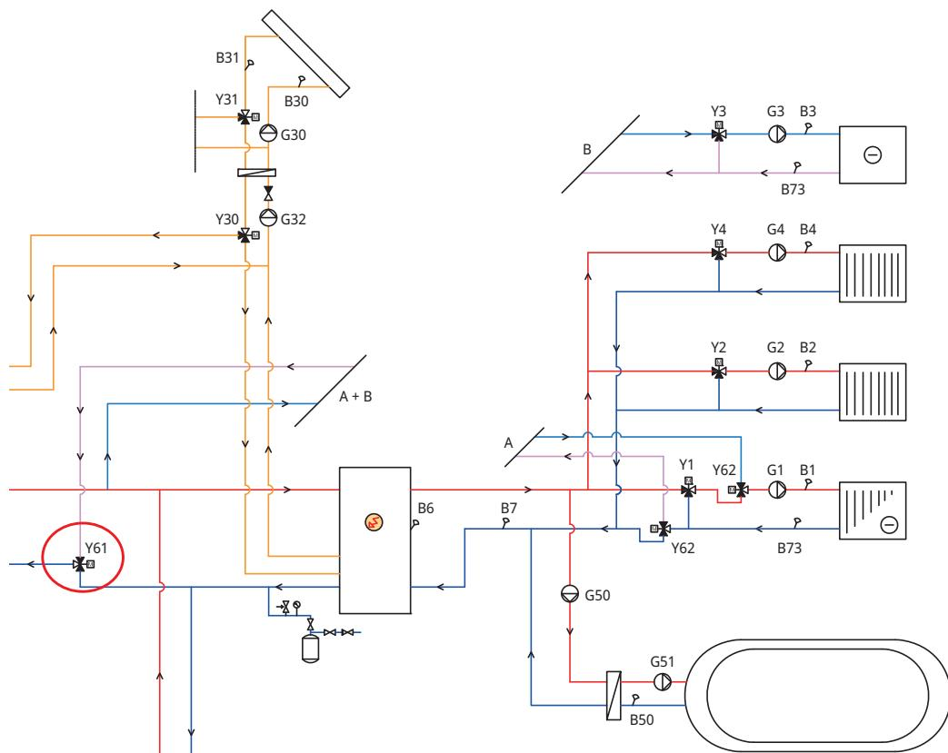
EcoLogic System 4/5 - Kjøletank mangler i systemet.
